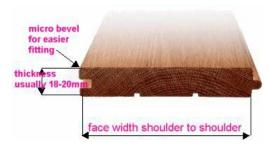
Solids are best secret nailed, with a portanailer machine (available for hire), or stuck to your sub floor using special adhesive. Generally narrower strips are more stable. Up to 83mm is described as strip and above 83mm as plank. Pre finished or pre lacquered saves considerable installing expense. The higher the grade the less colour variation and less knotting. Floors can be expected to last many lifetimes with
